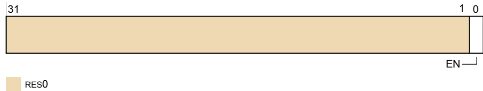
Figure D8-4 AMUSERENR_EL0 bit assignments
